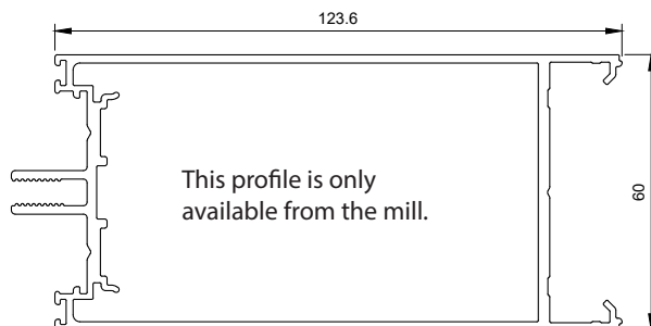
DIE No. W58660 F60 Transome Non Thermal 130mm
